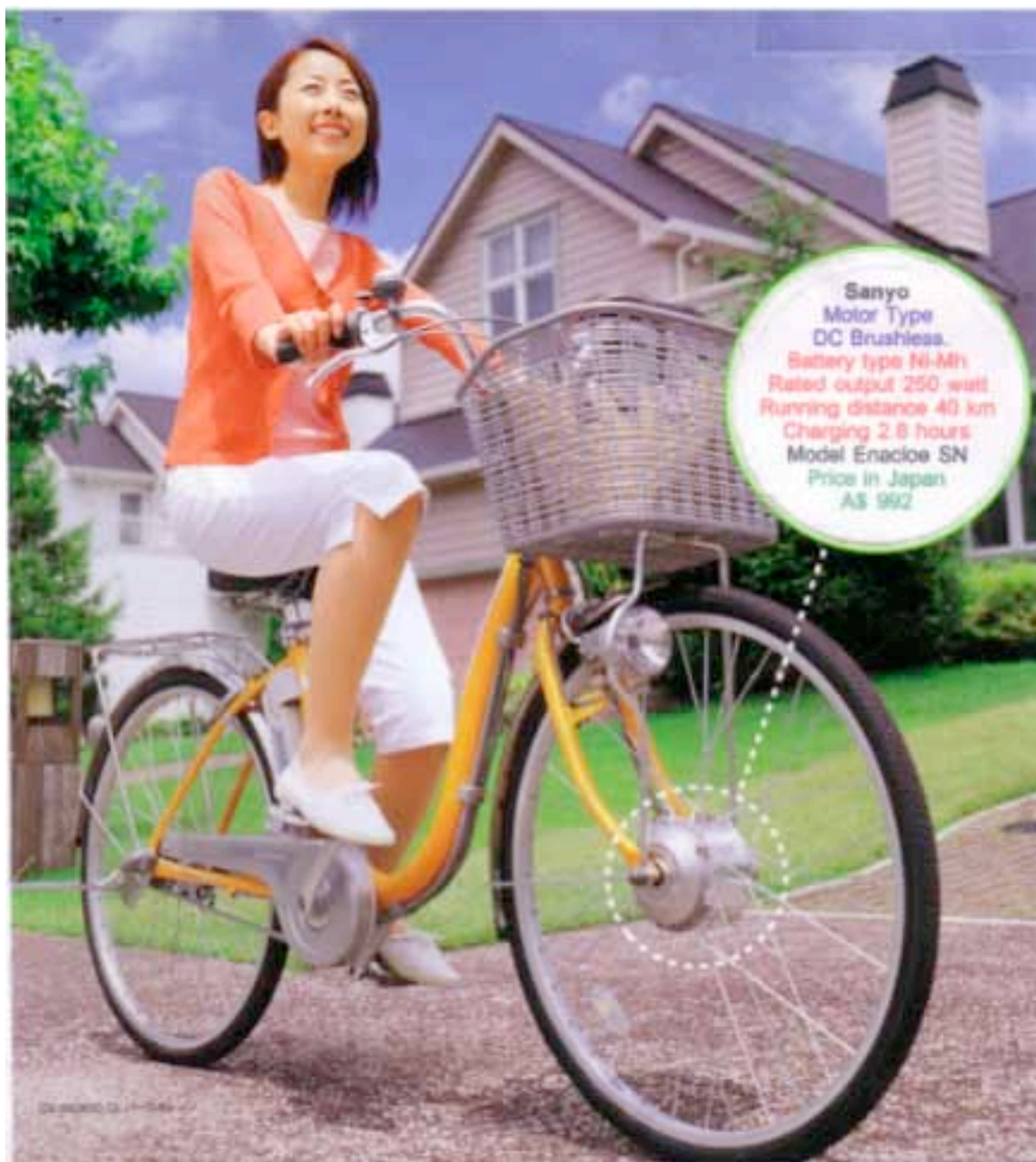
Figure 3. Japanese pedelec with ladies frame. Note the front wheel motor and small battery behind the riders right foot. It looks and rides like a bicycle as do most Japanese pedelecs sold in 2010 which also have Lithium batteries
