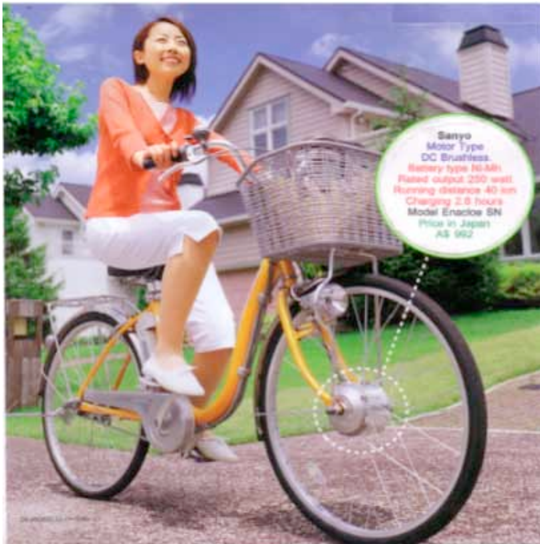
Figure 1. Japanese pedelec with ladies frame. Note the front wheel motor and small battery behind the riders right foot. It looks and rides like a bicycle as do most Japanese pedelecs sold in 2010 which also have Lithium batteries
