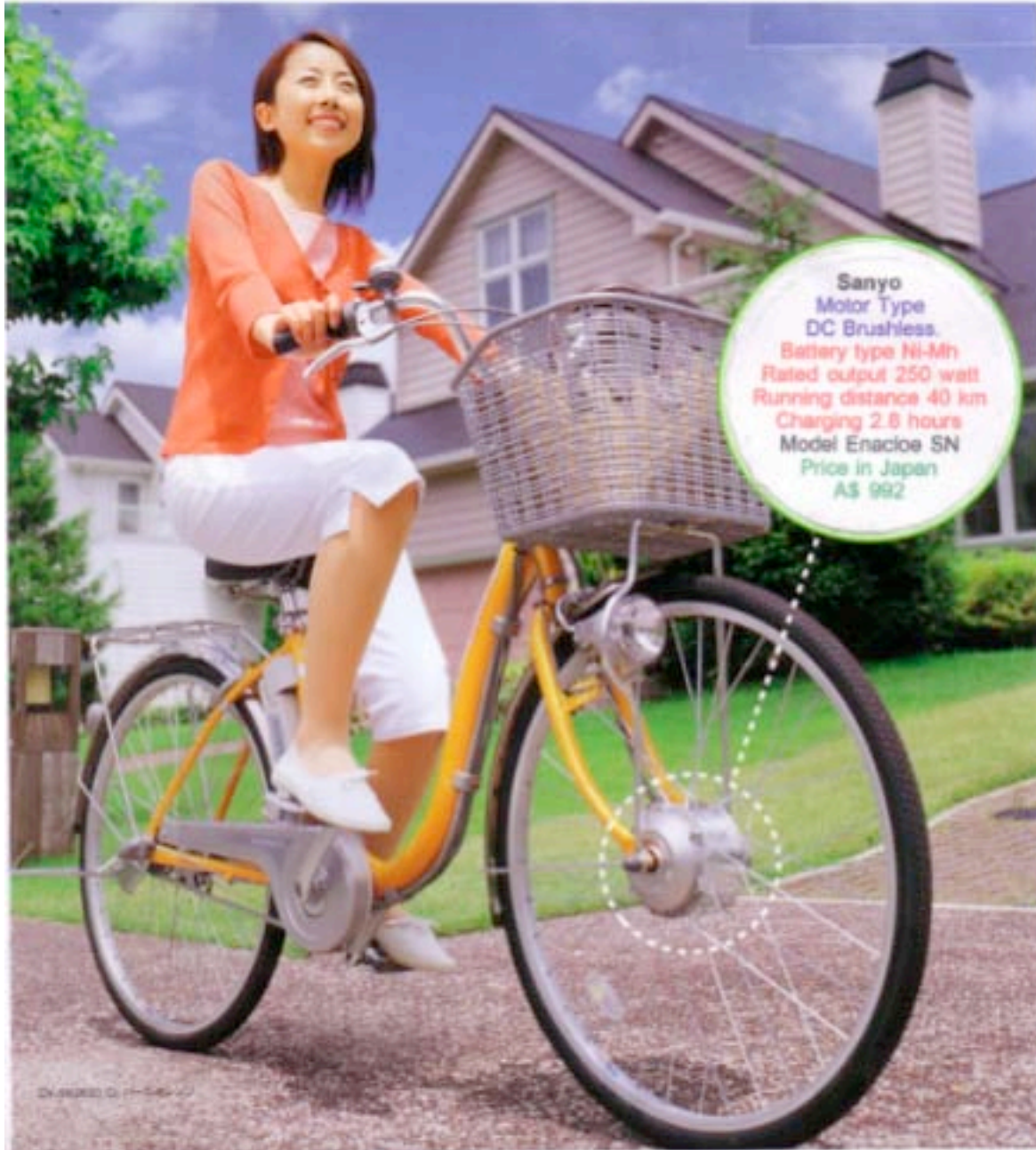
Figure 2. Japanese Pedelec with ladies frame. Note the front wheel motor and small battery behind the riders right foot. It looks and rides like a bicycle as do most Japanese Pedelecs
