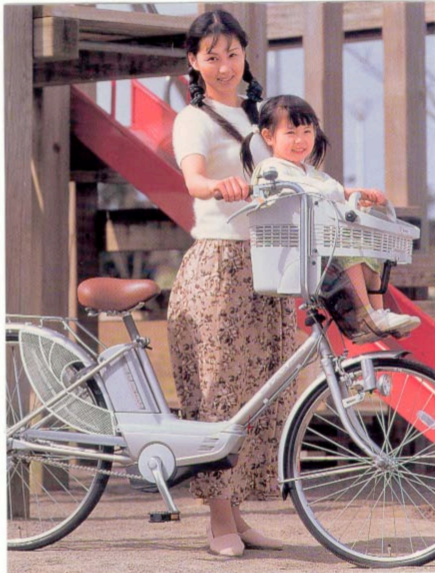
Figure 2. The PAS Little More has (1) a stable child seat, (2) ease of control and operation with a new keyless switch design and battery remaining indicator, (3) dynamo lighting control from handle bar mounted lever, (4) battery charging time of only 2.8 hours; on a single charge will travel 38 kms over flat roads. (5) It has a 3 speed integrated gear.
