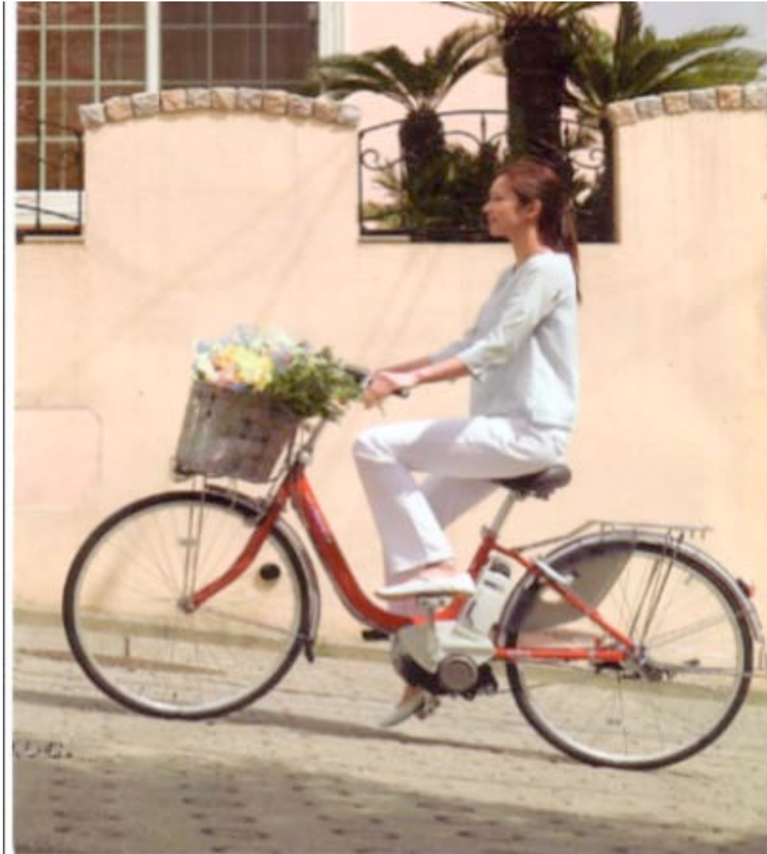
Figure 5 Shows an able bodied female around 55 kg in weight riding easily up hill. An overweight male of around 110 kg would stall the motor very quickly. This is why those with weight problems need a extra 150 watts more than the existing 200 watt maximum power output.
